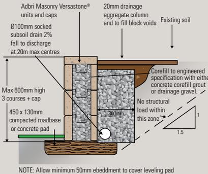
NOTE: Allow minimum 50mm ebeddment to cover leveling pad
