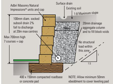
NOTE: Allow minimum 50mm ebeddment to cover leveling pad
