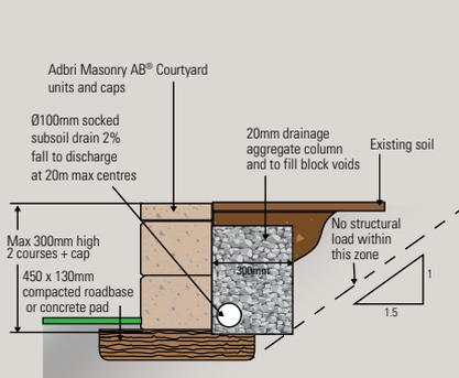
Max 300mm (2 units) high for gravity retaining walls. Build free standing walls to 750mm and piers to 900mm when not retaining.
