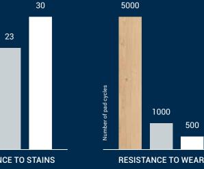
Wear resistance measurement based on Tarkett's internal tests (based on EN ISO 16094)
