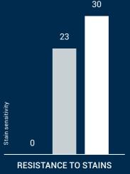
Stain resistance measurement based on Tarkett's internal tests (in compliance with ISO 26987).
