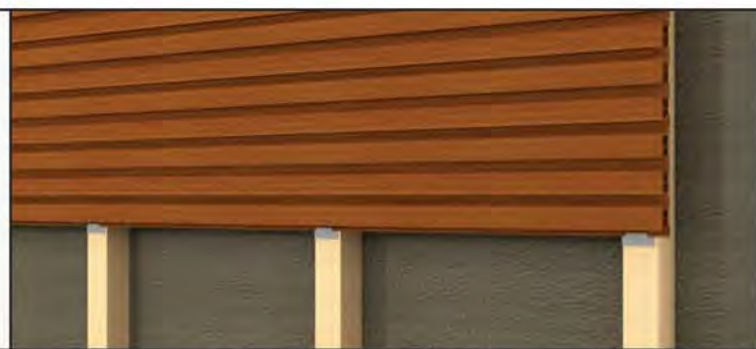
THO -26 Second Board Installation
