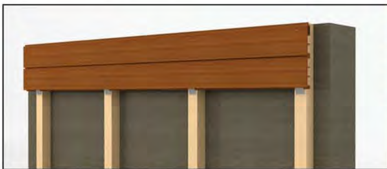
QBI-09 and QBO-16 Second Board Installation
