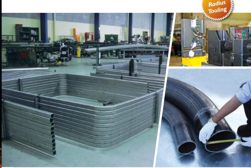
CNC Mandrel Bending is a highly specialised pipe bending process which gives the ability to produce tight radius bends with NO wrinkles or deformation.
