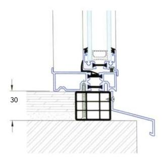
Window cill connector profile  $30 \times 37$  made of white plastic
