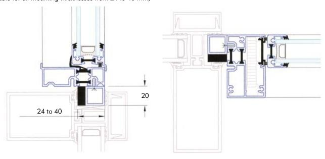
Installation in window frame and other glazing systems Adaptor profile  $30 \times 42$  mm (also available in  $30 \times 44$  and  $30 \times 48$ )
