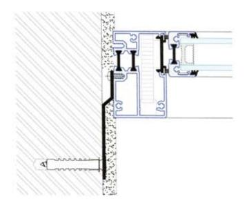
Assembly with masonry clip
