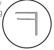
8. Pull the protective film back on the sides of the sheet and place the rubber gasket\* on both sides of the sheet to be inserted into the H Joiner. Then use either the F section (Barge ends) or the next H joiner on the side away from the secured H joiner. Insert this section on to the sheet and into the secured H joiner by tapping it in with a rubber mallet than secure the unsecured section as before.
