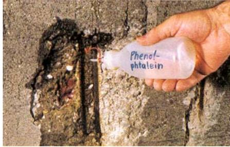
When phenolphthalein is sprayed onto concrete, only those areas with a pH value greater than 10 will turn pink. Other areas where the phenolphthalein remains colourless are therefore carbonated and should be removed during repair preparation.
