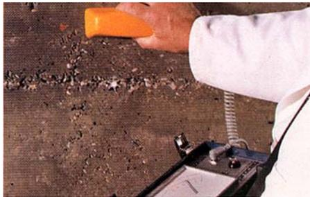
If the depth of the carbonation is known, then the rate at which it has occurred can be estimated for the year of construction. A cover metre will enable you to find the depth of cover over the reinforcing steel and therefore it is possible to calculate when the reinforcing steel itself will come under attack and expand through the overlying concrete.
