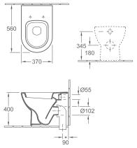
\*S-Trap wall-face pans supplied standard with 8712 vario bend to suit 90mm set out
