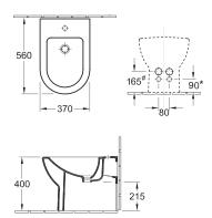
\*Hot/Cold Water Entry points need to be 40mm left & right of centre & 90mm from finished floor #Waste Outlet point needs to be 40mm left OR right of centre & 165mm from finished floor - Suitable for P-Trap Installation ONLY
