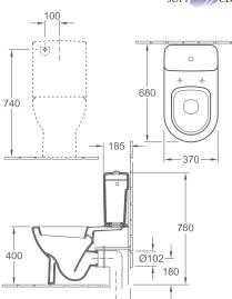
\*Recommended s-trap waste set-out 140mm (adjustment range 90-180mm)
