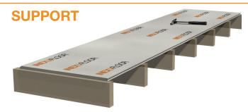
\*When using **INEX>FLOOR** as a substrate for floor tiling, if the tile size is greater than 300mm in any direction, floor joist spacing should be no greater than 450mm centres with an approved tile adhesive for both interior and exterior applications.
