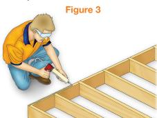
When fixing **INEX>FLOOR** to the joists it's good practice to apply a 6mm diameter bead of **INEX>BOND** to bond **INEX>FLOOR** to the frame even when mechanical fixings are used. This will fill any gaps arising from acceptable construction tolerances and minimise the possibility of a 'squeaky' floor developing as the floor ages.
