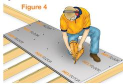
**Note:** Do not install the last row of fasteners adjacent to the tongue & groove joint until after the joint is completed.
