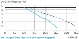
P1 - Output flow rate with one motor engaged OUTPUT P1 + P2 - Output flow rate with two motors engaged (litres/min)
