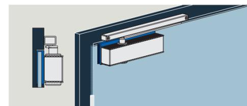
Mounting of glass clamping device
