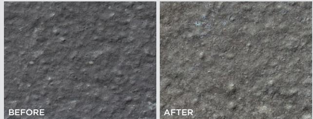
\* Product samples are independently tested in a NATA certified lab for 2,000 hours with cycles of UV exposure and condensation to simulate natural weather exposure. Testing has been performed on product samples of similar colour for fair comparison
