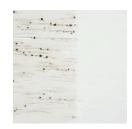
Conventional coating products were used on the left whilst the wood on the right was coated with Teknos antibleed primers
