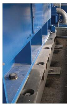
High flow, high strength, long working time natural aggregate grout with dual phase shrinkage compensation, ensures long term performance in all types of critical machinery grouting. This product sets the standard for natural aggregate precision grouts.
