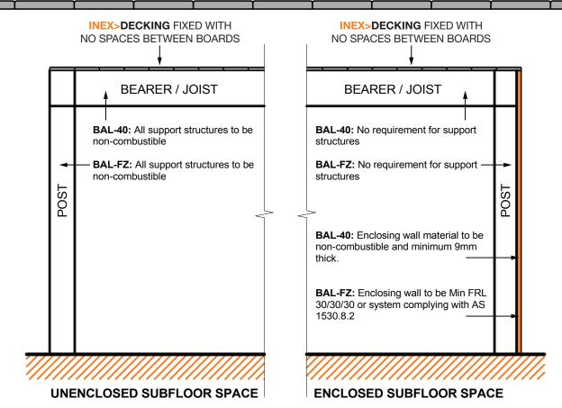
This diagram outlines the requirements under AS 3959-2009 Construction of buildings in bushfire-prone areas for the framing of verandas, decks, steps, ramps or landings for either BAL-40 or BAL-FZ construction.
