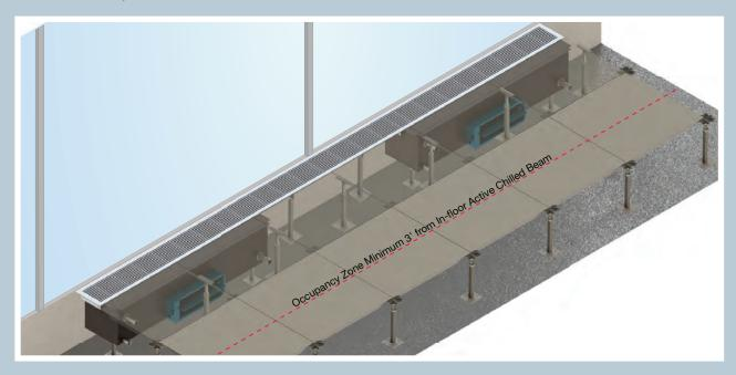
Segmented Design: In-floor Active Chilled Beams installed with raised floor panels and carpet between units.
