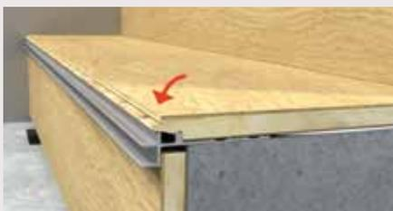
4. Place a plank on the step against the rising edge of the sub-profile.
