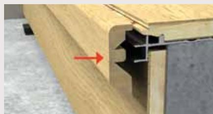
6. Press the Incizo® profile onto the sub-profile.
