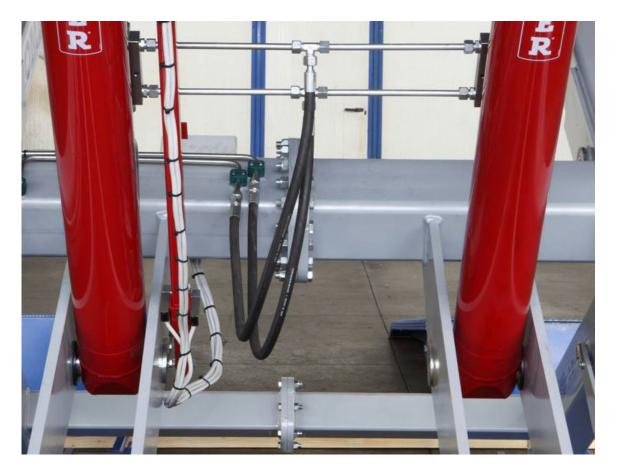
Heavy duty hydraulics allow maximum load lift. Built in valves for reading pressure differential and ensures safety which is a prime consideration.
