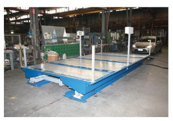
The platform is built with a series of galvanised panels which are both extremely sturdy and also light.
