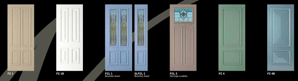
Description: Primed highly moisture resistant MDF faces, 38mm timber perimeter frame. All doors routered both sides and moulded one side. "B" in design code denotes raised panel to one face. \*Special sidelite width up to 550mm. Glazed doors are designed to be fitted with bead on inside. Trimming Recommendation: 5mm from top, bottom and each stile. For further technical information and glazing options refer to pages 38-39.
