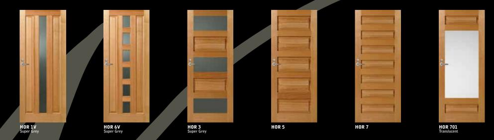
Description: Select hardwood, joinery door construction, square rebate to one side, bevelled bead to one side. In applications exposed to direct weather, hang door with bevelled bead to the outside. Includes 30mm fielded panels. Trimming Recommendation: 5mm from top, bottom and each stile. For further technical information and glazing options refer to pages 38-39.
