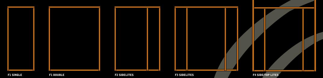
Description: Solid timber frame - 140mm x 40mm. All frames are made to have any glazing inline with the door (to the inside). Sill: Optional Merbau sill - 169mm x 40mm. Note: to suit 2040 x 820 door.
