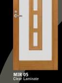
**Description**: Select hardwood, joinery door construction, stepped quad profile to one side, stepped quad loose bead to one side. In applications exposed to direct weather, hang door with stepped quad bead to the outside. **Glazing**: All glazing is to Australian Standard. Only flat surface glass can be used for Mirage range. **Trimming Recommendation**: 5mm from top, bottom and each stile. For further technical information and glazing options refer to pages 38-39.
