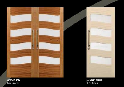
Description: Select hardwood, square rebate to one side, bevelled bead to one side. In applications exposed to direct weather, hang door with bevelled bead to the outside. Wave Paint is made from MR MDF and should be fitted with the glazing bead to the inside. Trimming Recommendation: 5mm from top, bottom and each stile. For further technical information and glazing options refer to pages 38-39.
