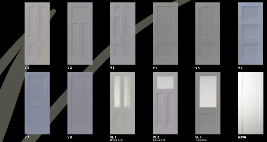
Description: Medium Density Fibreboard - 12mm MDF faces, solid construction, routered both sides. Has all the design benefits of a traditional door but eliminates the potential problems of shrinkage, movement and gaps. Note: Other rout profiles and pre-hung available, POA. Also available in bi-Fold. Trimming Recommendation: 5mm from top, bottom and each stile. For further technical information and glazing options refer to pages 38-39.
