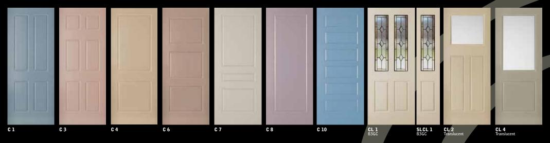
Description: Medium Density Fibreboard - 12mm MDF semi solid construction, featuring square corner rout to both sides. Glazed doors are designed to be fitted with bead on inside. Note: Other rout profiles and pre-hung available, POA. \*Special sidelite width up to 550mm. Trimming Recommendation: 5mm from top, bottom and each stile. For further technical information and glazing options refer to pages 38-39.
