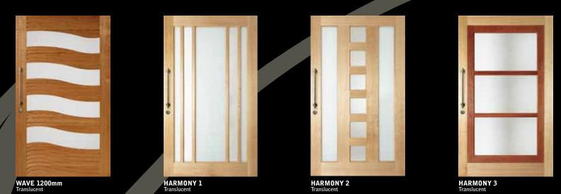
**Description :** Select KD hardwood, square rebate to one side bevelled bead to one side. In applications exposed to direct weather, hang door with bevelled bead to outside. Harmony 3 is a select hardwood frame with an internal Jarrah frame laminated to it, highlighting the contrast of the two timbers. **Trimming Recommendation**: 5mm from top, bottom and each stile. For further technical information and glazing options refer to pages 38-39.
