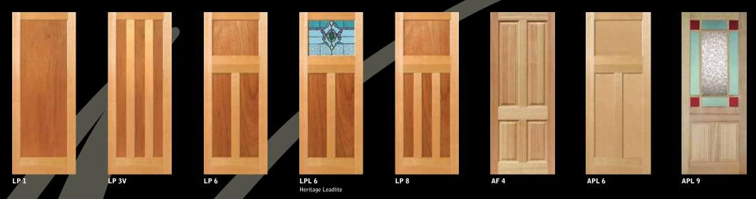
Description: Select hardwood with Lauan plywood panels for stain or clear finish. Available in MDF for a paint finish. AF4 has 20mm fielded panels. APL9 has Victorian Ash panels and insertion moulds. Glazing for these doors is POA. Trimming Recommendation: 5mm from top, bottom and each stile. For further technical information and glazing options refer to pages 38-39.
