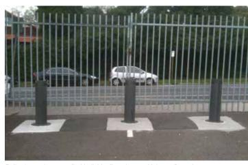
Bollards can be controlled individually or in a multiple configuration
