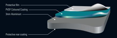
The material is rigid, resistant to blows, breakage and pressure and has high bending, buckling and breaking strengths.
