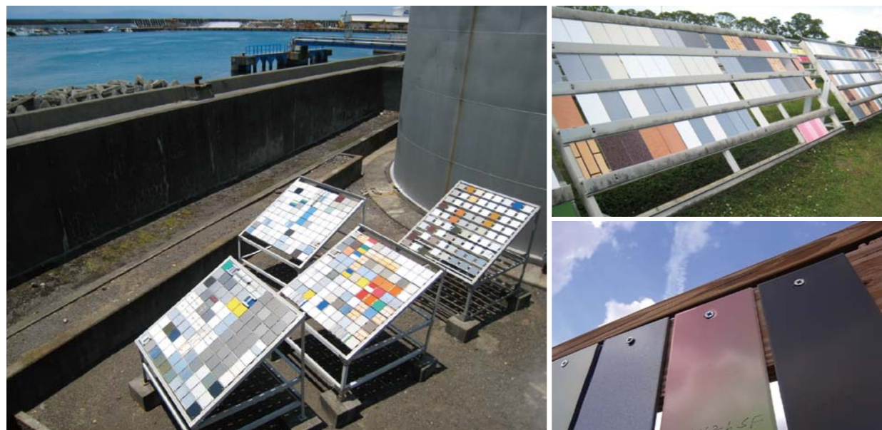
Natural exposure test in Japan & South Florida, USA
