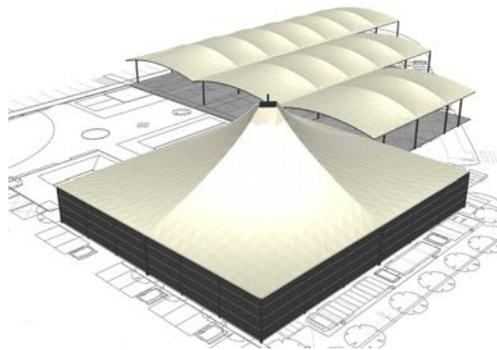
The most common tensile membrane roof shapes feature barrel-vault or conical geometries, although with flexible architectural membranes, there are limitless possibilities to the shapes that can be created.
