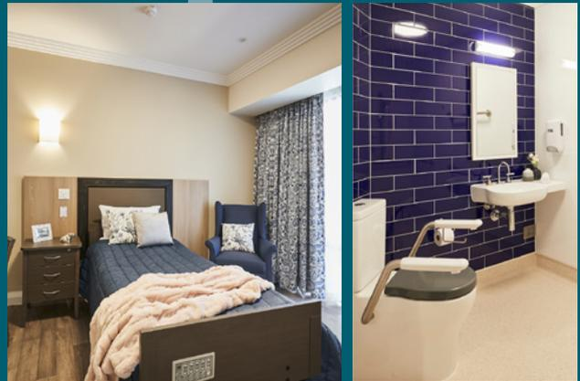
The basins are equipped with Elegance lever basin tapware, which combines familiar shape and contemporary design with hot, cold & warm coloured indicators for better visibility. The tapware also features extended levers to give users with limited hand mobility a comfortable grip on the handle. The range was installed in the showers alongside Caroma's Plus Starsafe II care product too.
