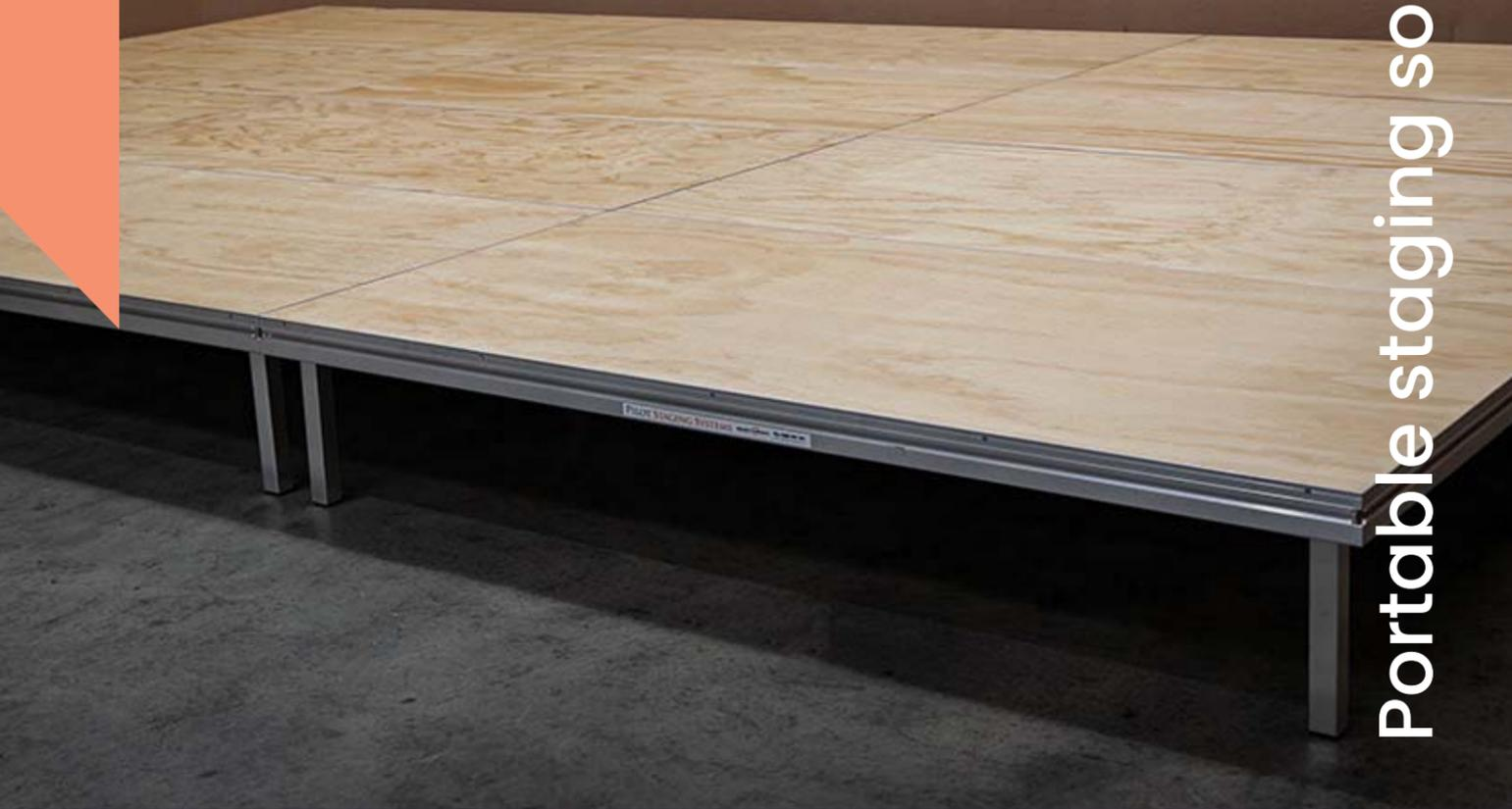
**Operation:** Aluminium legs are placed in the corner brackets and wing nuts tightened by hand. The leg is securely held in the corner with a sliding T piece. Podiums are attached together with a hand tightened Klemm-fix connector. Accessories are attached to the podium aluminium extrusion using T bolts, and hand wheels are finger tightened.
