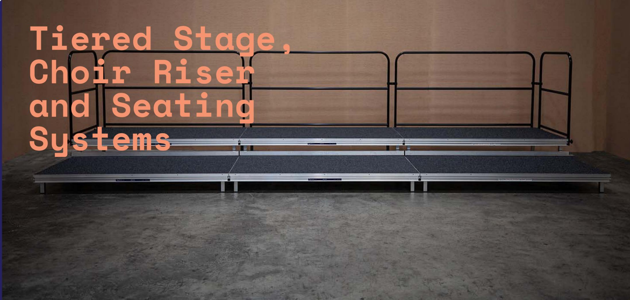
Our modular podium systems adapt easily from single to multi-level by changing the leg lengths in the corner castings. The unique Klemm-fix connector joins each level securely, and leg clamps secure the multiple levels to one other. We can design a tiered stage to suit your requirements, and as the entire system is free standing, it will accommodate unusual wall shapes and obstacles.
