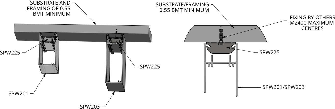
Slab edge fixing details with expansion joint
