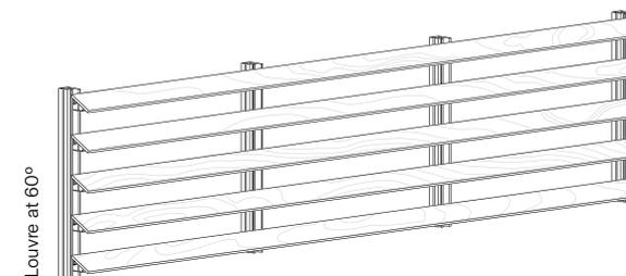
The NATURCLAD-W installation system in fixed louvre mode enables slats to be installed at 0°, 30° and 60°, both horizontally and vertically.
