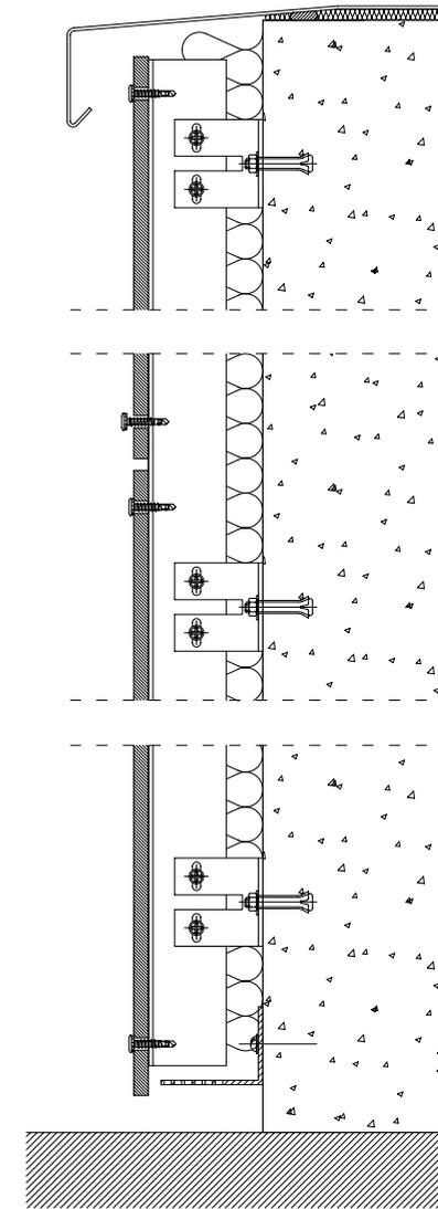
The ventilated façade is an efficient bioclimatic architecture solution that provides thermal insulation. In other words, it reduces heat dissipation in the cold months and heat absorption in the warmer months, resulting in a marked improvement in comfort inside the building.
