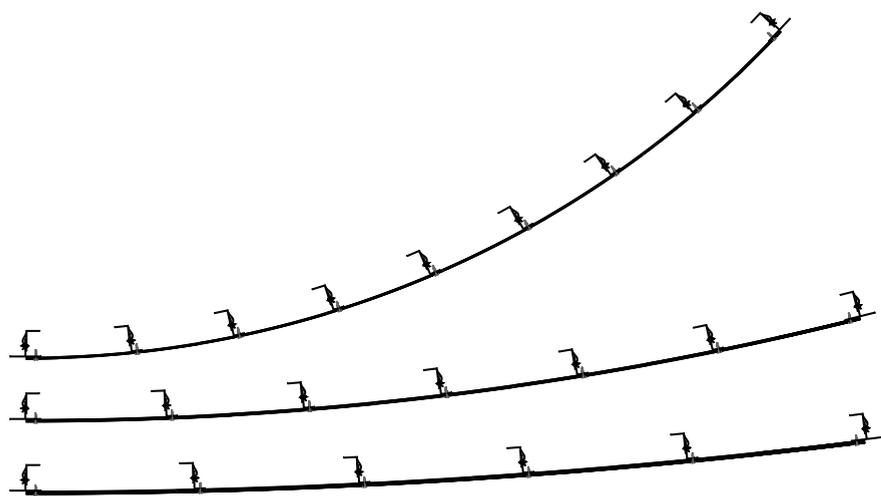
The flexibility of the wood fibres allows NATURCLAD-W panels to adapt to certain radii of curvature, whether concave or convex.
