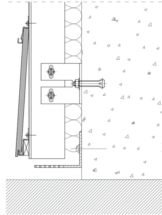
The overlapping slats system enables a range of assembly procedures without needing to change the position of the parts' profiles.
