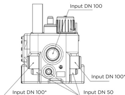
\*This entrance must be directed at a height of 250 mm above the ground level directly after the lifting station.
