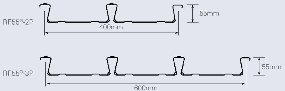
RF55® is manufactured from G550 (550 MPa Yield Stress) DECKFORM® steel with a Base Metal Thickness (BMT) of 0.60mm, 0.75mm, and 1.00mm. The thicknesses of 0.90mm and 1.20mm BMT are also available on request. The galvanised coating thickness is a Z350 (350 g/m<sup>2</sup>) in accordance with AS 1397:2001.
