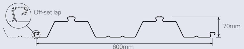
KF70® is manufactured from G550 (550 MPa Yield Stress) DECKFORM® steel with a Base Metal Thickness (BMT) of 0.75mm and 1.00mm. A thickness of 0.60mm BMT is also available upon request, subject to stock availability and order quantities. The galvanised coating thickness is a Z350 (350 g/m<sup>2</sup>) in accordance with AS 1397:2001.
