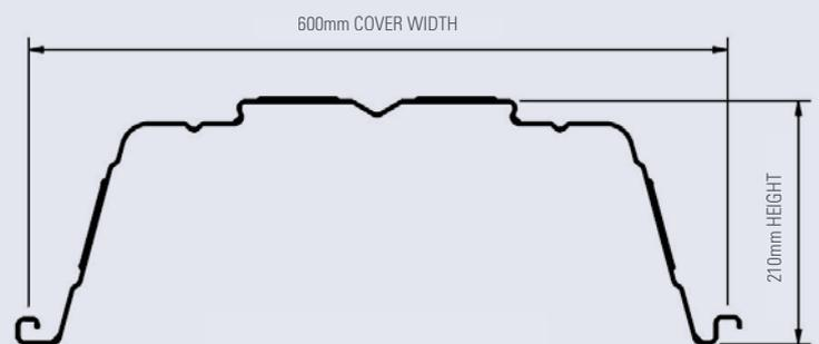
KingFlor® SlimDek 210™ decking is manufactured as standard from either G550 (550MPa Yield Strength) 1.0mm Base Metal Thickness (BMT), G500 1.2mm BMT or G500 1.5mm steel. The galvanised coating thickness for all three is Z350 (minimum 350g/m<sup>2</sup>) in accordance with AS 1397-2011.
