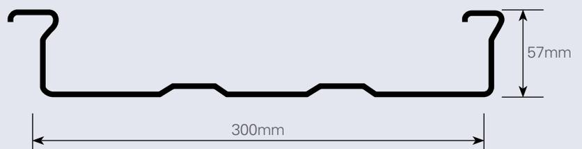
KF57® is manufactured from G550 (550 MPa Yield Stress) DECKFORM® steel with a Base Metal Thickness (BMT) of 0.60mm, 0.75mm and 1.00mm. The galvanised coating thickness is a Z350 (350 g/m<sup>2</sup>) in accordance with AS 1397:2001.
