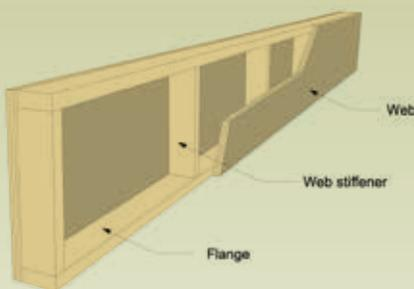
***Flexible and lightweight, plywood box beams are a high-strength timber product that can be used in a vast range of residential, industrial and commercial design and building projects.***
