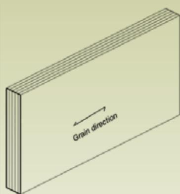
**The biggest advantage of LVL is the fact that it is manufactured continuously, meaning it is available in almost any length.**
