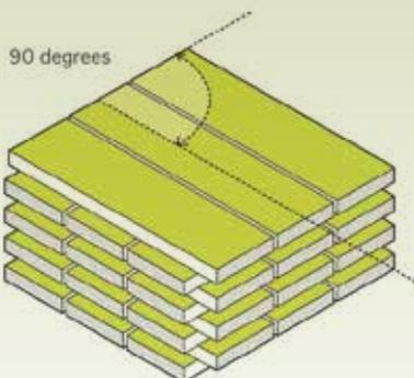
**Cross laminated timber (CLT) is an engineered wood product for the future, making the construction of entire mid to high rise buildings from timber a reality - an elegant solution for the building industry as it pursues more sustainable building practices.**
