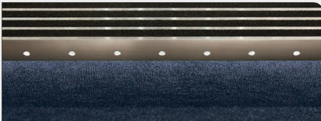
**DEC Series.** 6mm visual holes at approximately 66mm centres allow the LED's to be seen in the riser of the nosing, whilst also fan lighting the riser and the tread below.
