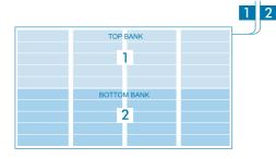
that all blades in the top halves of all the bays form a bank and operate simultaneously and all the blades in the lower halves of all the bays form a second bank and operate simultaneously. However, various switching and wiring configurations allow multiple windows to be controlled simultaneously or independently depending on individual preferences.
