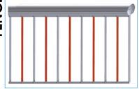
A fence is often used to stop pedestrians gaining entry under the boom pole. In areas where there are numerous pedestrians it is advisable to also fit a warning device such as a buzzer or flashing light.
