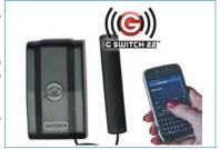
GSM MOBILE PHONE CONTROL: The G Switch module can be programed to accept up to 500 different mobile numbers. When the module receives a call from a registered mobile it will open the boom gate but does not incur any call charges.
