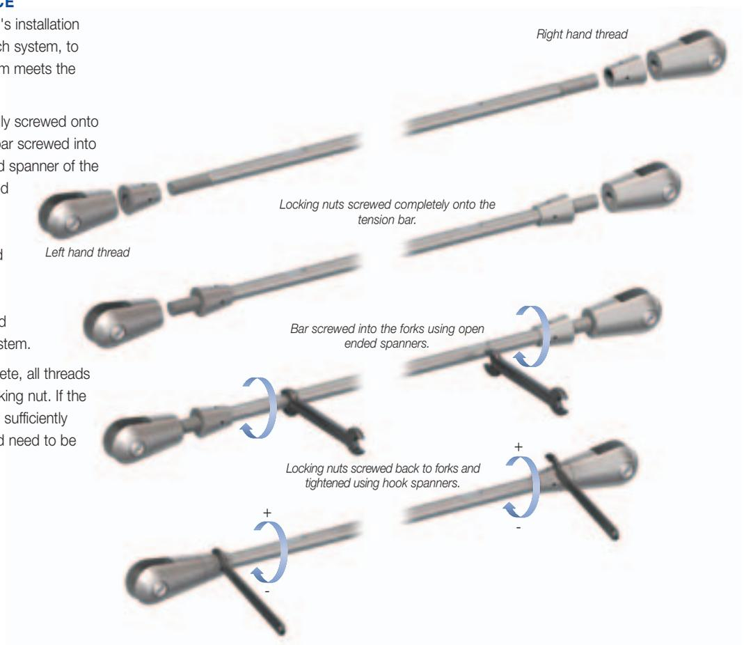
Each fork is supplied with a locking nut and pin to enable fixing to a connecting plate or anchor disc. The installation requires a twin-pin driver. Two driver bits of the appropriate size are supplied with each Ancon system. This type of fixing, known as 'Snake Eyes'\*, allows a high torque to be achieved without damage to the pin.
