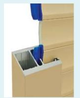
Manufactured from 41mm roll formed aluminium with a polyurethane foam core and a heavy duty Maxiblock® 70mm track with built-in internal locking chamber.
