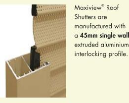
TECHNICAL INFORMATION Maximum width - 5 metres Track sizes - 63mm standard Colour range - Standard and customised colours available Profile - Perforated and non-perforated.
