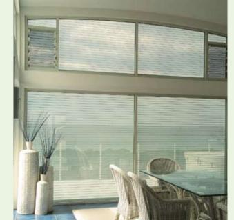
Blockout's Maxiview Standard perforated option achieves external visibility through 54,000 perforations per square metre in the shutter profile. The perforations are only 19% of the overall shutter profile (curtain), therefore glare, heat gain and heat loss are still reduced.
