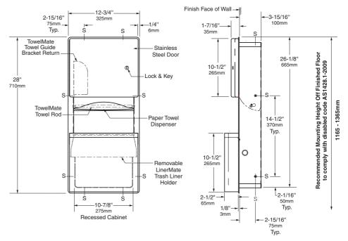
Rough Wall Opening 11-3/8" (290mm) wide 26-5/8" (675mm) high 4" (100mm) minimum recessed depth
