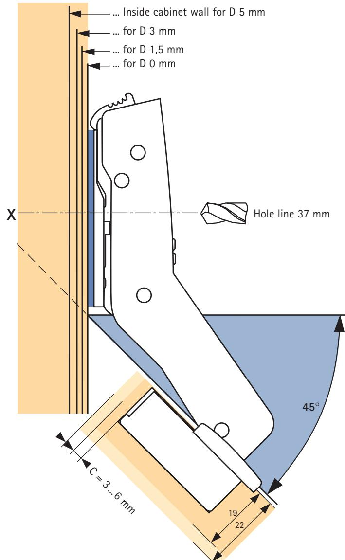
**Fast-assembly concealed hinge with integrated soft-close function
