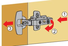
Characteristic for sensys hinges is the ergonomical snap-on assembly. The hinge is slipped into the front of the mounting plate ①, then a light finger pressure and the hinge arm latches onto the mounting plate ② with an audible click.
