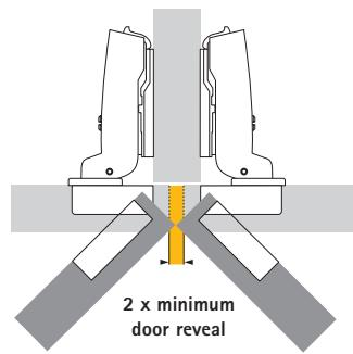
For half overlay configurations, the total reveal between the doors must be chosen to correspond to twice the door reveal. Both doors can then be opened at the same time.
