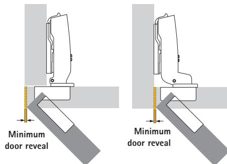
The minimum reveal (also known as the minimum clearance) is the space required at the side so that the door can open. The size of the minimum reveal depends on the cup distance C, the door thickness and the type of hinge selected. Radii on the door edges reduce the minimum clearance. The required minimum reveal is shown in the table for the respective hinge types.
