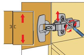
Using height-adjustable mounting plates makes it possible to align the exact door height.
