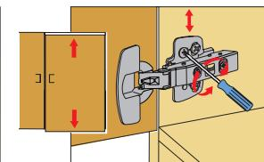
Direct, variable height adjustment with eccentric screw
