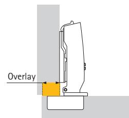
The overlay is the distance by which the door projects over the cabinet front.
