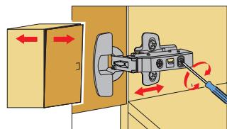
Direct, infinitely variable depth adjustment
