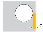
The larger the cup distance, the smaller the required minimum reveal.
