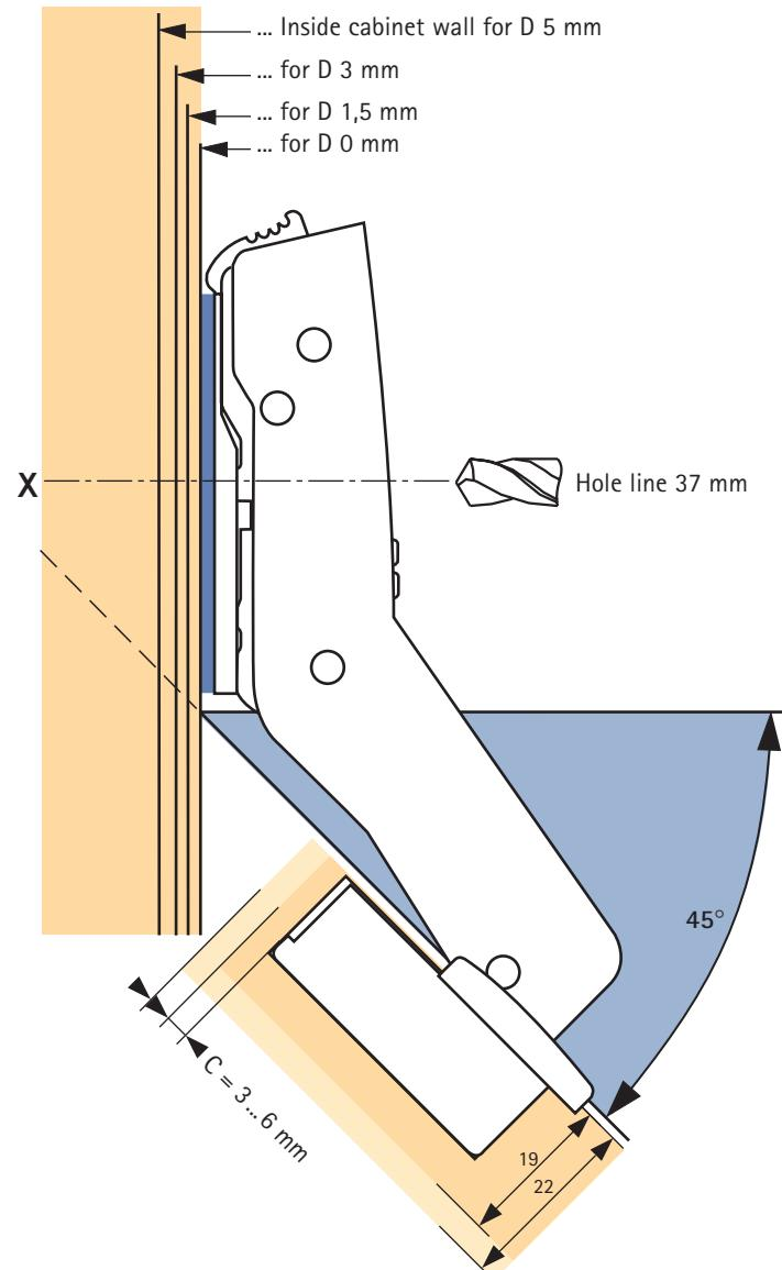
**Fast-assembly concealed hinge with integrated soft-close function
