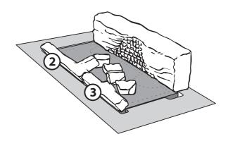
3. LOCATE LOG NO'S 2 & 3: Two front log no's. 2 and 3 are supplied to fit into the space between the metal frame and the ceramic base. These logs do not cover the front burner ports but are designed to deflect the front flame back into the fire.
