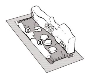
3. LOCATE LOG NO'S 2 & 3: Two front log NO'S. 2 & 3 are supplied to fit into the space between the metal frame and the ceramic base. These logs do not cover the front burner ports but are designed to deflect the front flame back into the fire.
