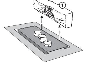
2. LOCATE LOG NO. I: This is the largest log that is positioned at the rear of the grate. Two locating pins are positioned at the rear of the burner. The large log has two holes on the underside to position in place.
