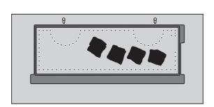
I. LOCATE 4 CERAMIC COALS: Four ceramic coals are supplied with the burner base. These coals must be laid in the position indicated on the drawing with the taller coals on the ends and smaller coals in-between.
