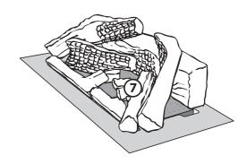
6. LOCATE LOG NO. 7: The charred effect of the log is positioned on the smaller coal in the centre of the burner on the right hand side.
