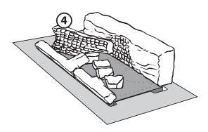
4. LOCATE LOG NO. 4. This log is placed with the thinner edge on the smaller coal. The charred effect is facing towards the front of the burner. The whole log is positioned on the burner base.
