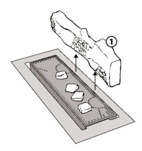
2. LOCATE LOG NO. I: This is the largest log that is positioned at the rear of the grate. Two locating pins are positioned at the rear of the burner. The large log has two holes on the underside to position in place.
