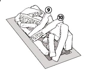
6. LOCATE LOG NO. 9. This log is placed on the rear log in the centre of the burner. Charred effect facing toward the left of the burner. The front rests on logs 2 & 3 on the join.
