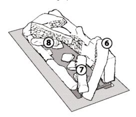
5. LOCATE LOG NO. 6. Place this log on the right hand side of the burner on the rear log in front of the pilot. Charred end facing inwards. The left hand side of the log is positioned between the metal uprights on the side of the grate.
