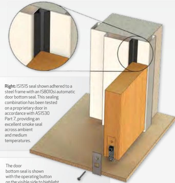
**Right:** IS1515 seal shown adhered to a steel frame with an IS8010si automatic door bottom seal. This sealing combination has been tested on a proprietary door in accordance with AS1530 Part 7, providing an excellent smoke seal across ambient and medium temperatures.
