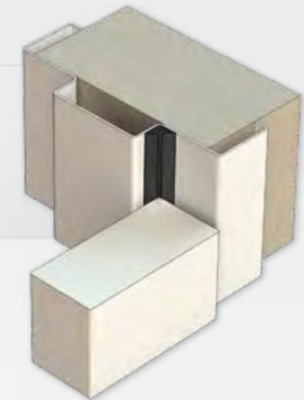
**Right:** IS1212 seal shown adhered to a metal frame. The symmetrical design of this seal ensures the fins are always in contact with two surfaces of the door leaf, creating an air chamber to provide excellent smoke and acoustic performance.
