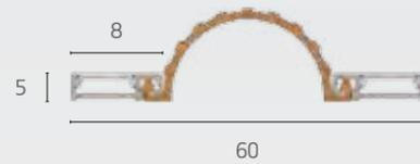
IS9050 Finger Guard Seal - hinge position
