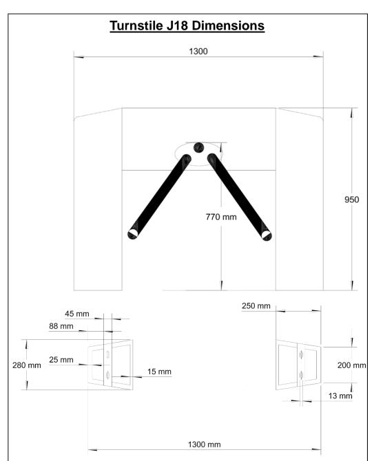
**NOTE:** The concrete pad should be 20Mpa (min) 150 mm thick, cured for 7 days on a suitably compacted foundation. Hold down anchors (4) to be 12mm dia x 100mm into the concrete.
