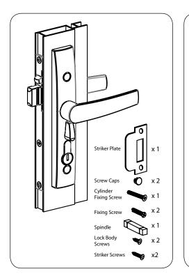
After sliding the Lock Body into the door cutout fasten with the two self tapping screws provided.
