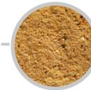
Fine cast of sand applied by air compressor sanding gun to assist with slip resistance
