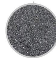
150mm compacted porous road base. 20/4mm graded material for compaction, with limited fines to maintain porosity. Installed in 3 layers of 50mm to ensure maximum compaction to 98%
