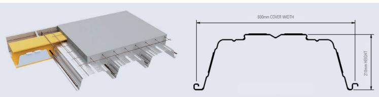
KingFlor® SlimDek 210™ decking is manufactured as standard from either G550 (550MPa Yield Strength) 1.0mm Base Metal Thickness (BMT), G500 1.2mm BMT or G500 1.5mm steel. The galvanised coating thickness for all three is Z350 (minimum 350g/m²) in accordance with AS 1397-2011.
