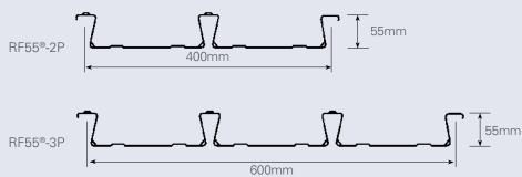
RF55® is manufactured from G550 (550 MPa Yield Stress) DECKFORM® steel with a Base MetalThickness (BMT) of 0.60mm, 0.75mm, and 1.00mm. The thicknesses of 0.90mm and 1.20mm BMT are also available on request. The galvanised coating thickness is a Z350 (350 g/m2) in accordance with AS 1397:2001.
