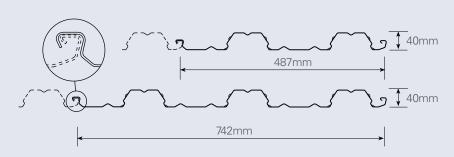
KF40® is manufactured from G550 (550 MPa Yield Stress) DECKFORM® steel in a 2 pan or 3 pan profile\* with a Base MetalThickness (BMT) of 0.60mm, 0.75mm and 1.00mm. The galvanised coating thickness is a Z350 (350 g/m2) in accordance with AS 1397:2001.
