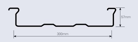
KF57® is manufactured from G550 (550 MPa Yield Stress) DECKFORM® steel with a Base Metal Thickness (BMT) of 0.60mm, 0.75mm and 1.00mm. The galvanised coating thickness is a Z350 (350 g/m2) in accordance with AS 1397:2001.
