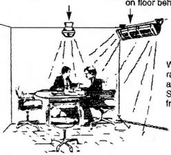
Warm floor reradiates heat. Warm air rises from floor. Some heat reflects from floor.
