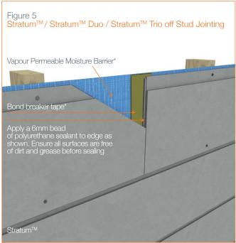
Off stud joining is suitable up to N3 Wind Zone only.
