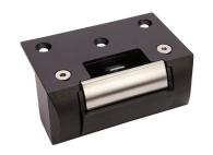
The RIM-Mounted, FES15 Series electric door strikes are designed for residential or light commercial applications where a rim mounted strike is required, such as pedestrian gates.
