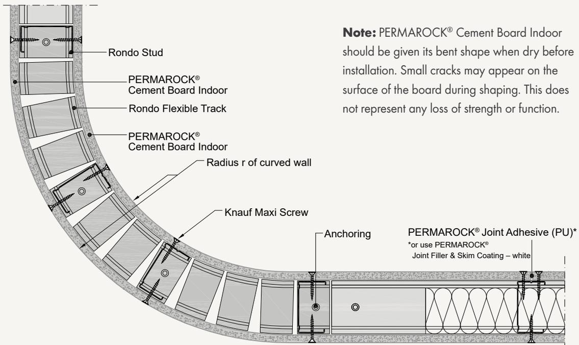
**Note:** PERMAROCK® Cement Board Indoor should be given its bent shape when dry before installation. Small cracks may appear on the surface of the board during shaping. This does not represent any loss of strength or function.
