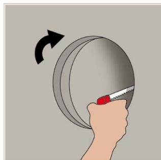
To make cut-outs for wiring and pipes, use a jigsaw or hole saw.
