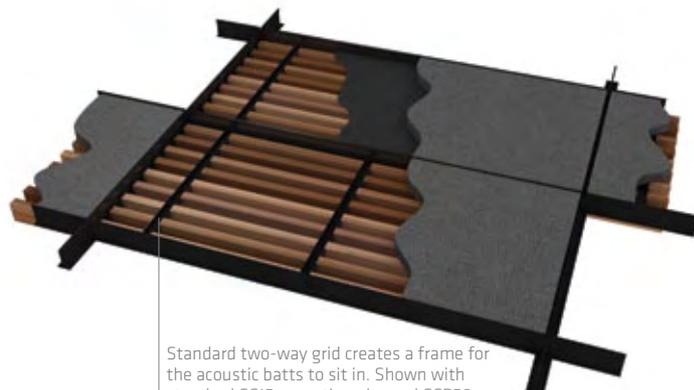
Standard two-way grid creates a frame for the acoustic batts to sit in. Shown with standard SC15 acoustic scrim and SCP50 acoustic polyester backing.
