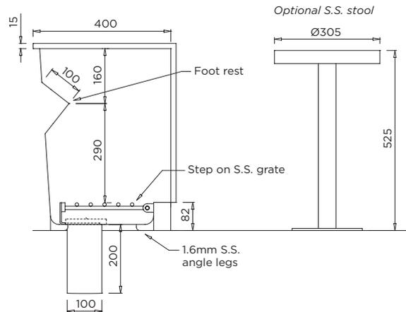
**MODEL TWUDU** Section: Floor Mounted Model
