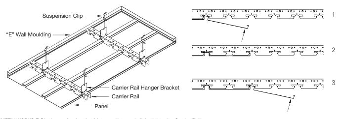
METALWORKS F-Plank are simply raised into position and clicked into the Carrier Rail.
